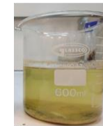
Collected Effluent after MBBR
