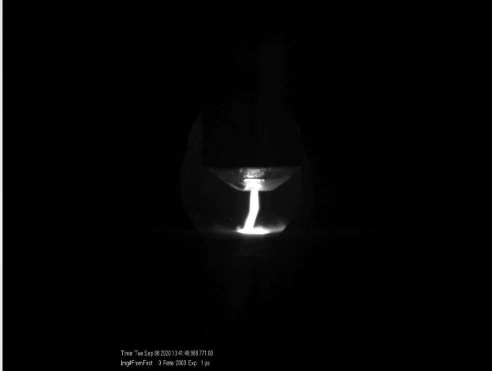
Fig.5. Visualization of the burning electric arc of the plasma torch. 1 - ignition, 2 – after 10 min. of waste recycling.
