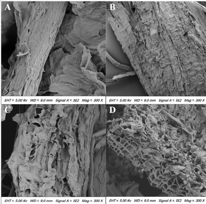
**Fig. 4.** Electron microscopy images of the micro structure of the mulberry bark samples treated with different enzymes. (A) Buffer treatment for 24 h (B) M137E/N269G alone (C) Cellulase alone (D) mixture of M137E/N269G and cellulase
