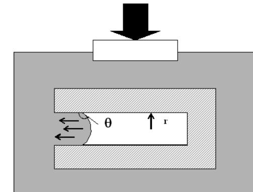
**During this process, mechanical energy is converted into interfacial energy**
