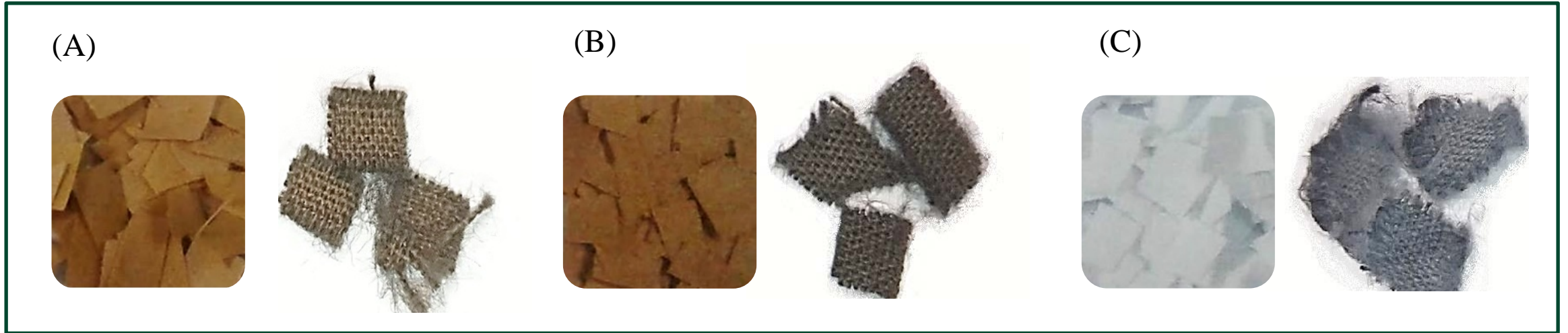
SupFig 2. WCotton pictures before (left) and after (right) dye adsorption (A) Fe007 in pH10, (B) Fe014 in pH10, (C) Pure Cotton in pH 2.5
