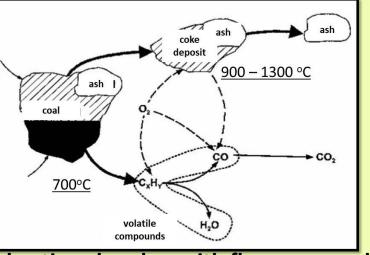
Fly ash is a fine 1-500µm fraction, which leaves a combustion chamber with flue gases and is collected in dedusting instalation using an electroprecipitator.
