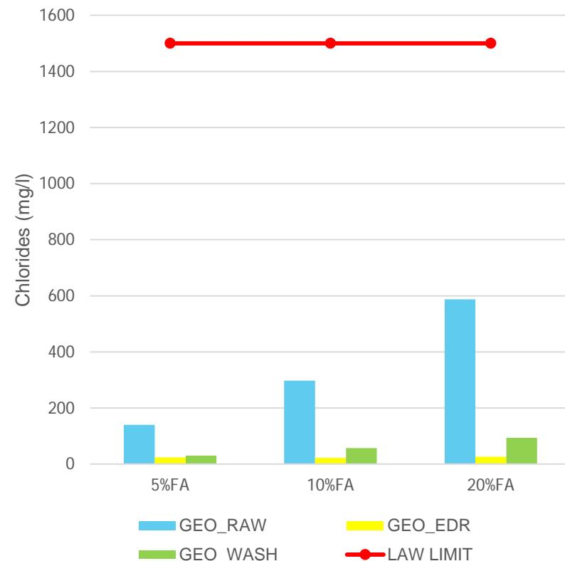
**Chlorides leaching** after 7 and 31 days of curing (Monolithic samples – EN12457 leaching test)
