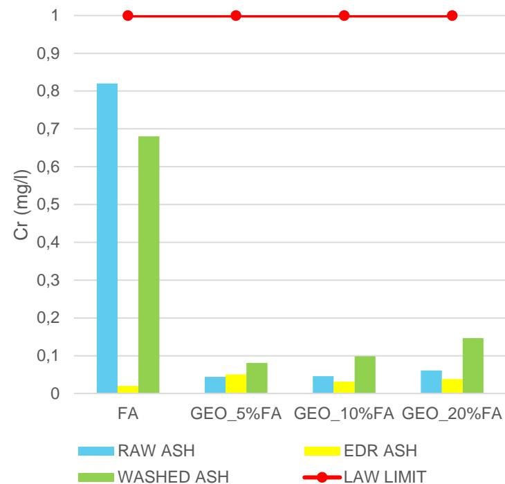
**Cr leaching** after 7 and 31 days of curing (Monolithic samples – EN12457 leaching test)
