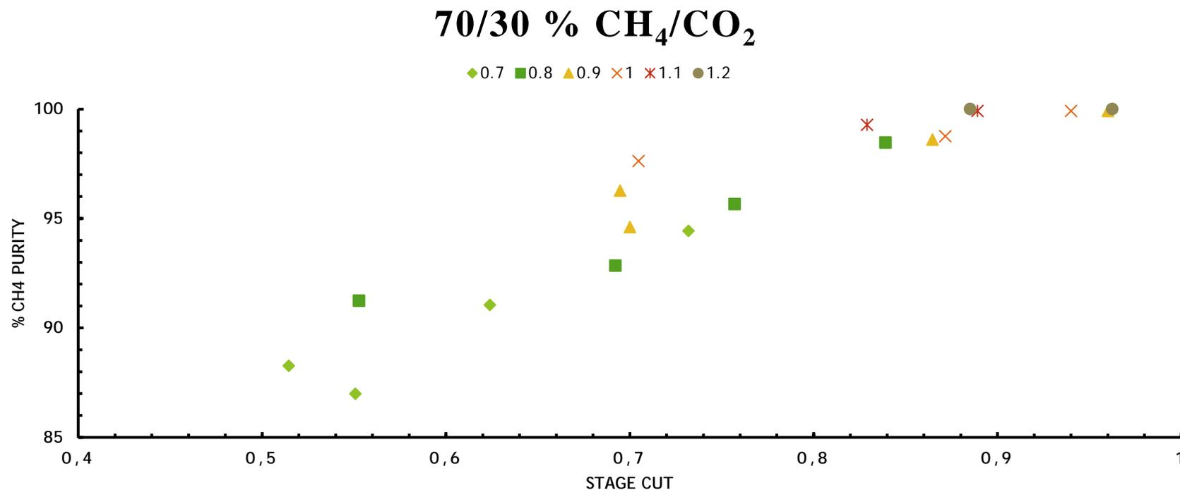
Increase of stage cut values leads to higher CH<sub>4</sub> purity.
