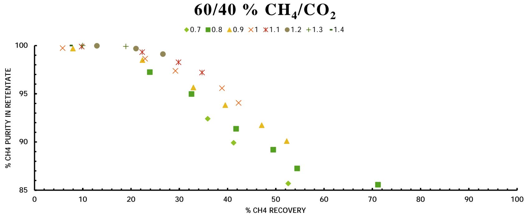
Increase of CH<sub>4</sub> purity when CH<sub>4</sub> recovery reduces.
