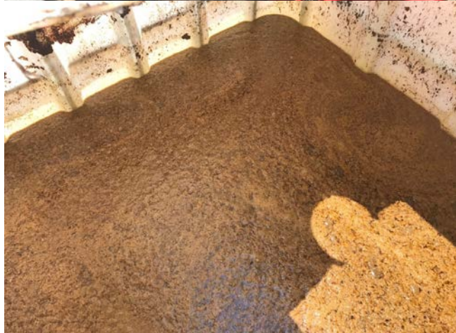
* Slurry after OFMSW squeezing
