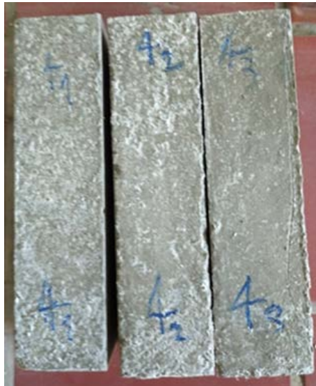
Reference sample without expansion (Left), semiconductor (SC) sample with air bubbles and expansion (Right)
