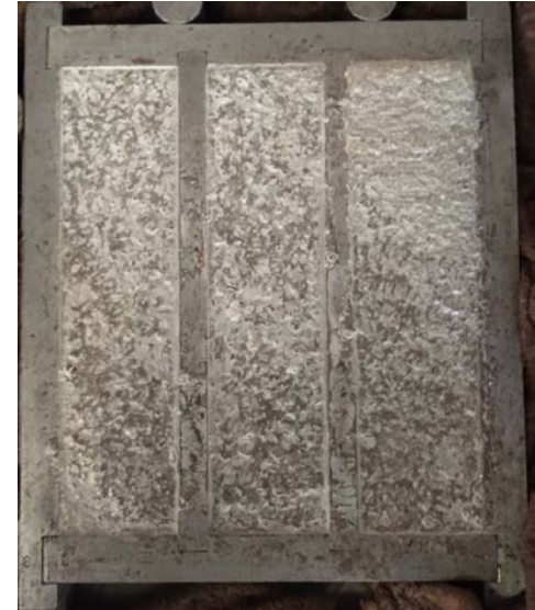
Prismatic mortars in the mold
