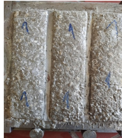
Reference sample without expansion (Left), semiconductor (SC) sample with air bubbles and expansion (Right)
