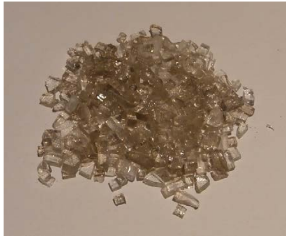
Glass particles > 2000 \mu\text{m} fraction mass: 85% w/w
