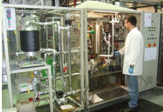
Small-scale catalytic hydrotreatment pilot unit
