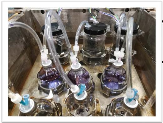
Biogas was collected through water displacement.
