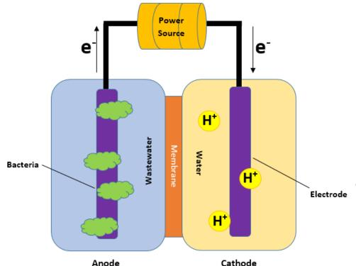
A (MEC) is a biological device capable of covert organic material into CO<sub>2</sub> and hydrogen (H<sub>2</sub>), along with free electrons by electrochemically active microorganisms.
