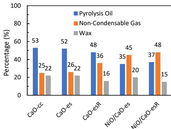
Figure 2. The effect of synthesized catalysts on pyrolysis of HDPE.
