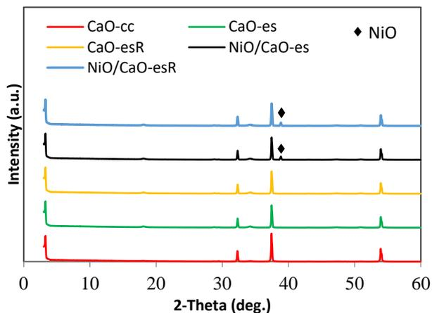
Figure 1. XRD results of synthesized catalysts.
