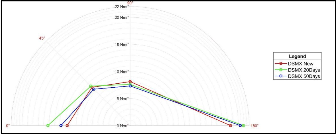
Fig.3 Flexural stiffness at different angles for new (t 0 ) and used (t 20 and t 50 ) ski boots.
