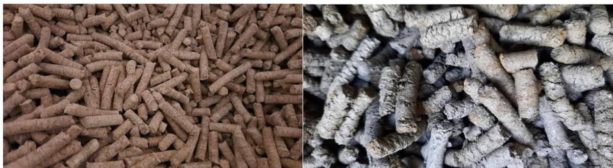
Fig. 1. Left: pelletized dried food waste as feedstock before TP, right: SCP/biochar after TP.
