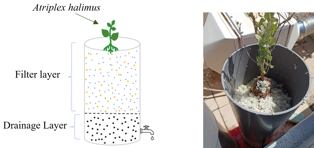
Fig. 1.: a) Schematic presentation of VFCWs used in experimental studies, b) VFCW filled with the mixture perlite and sponge cubic form carriers.
