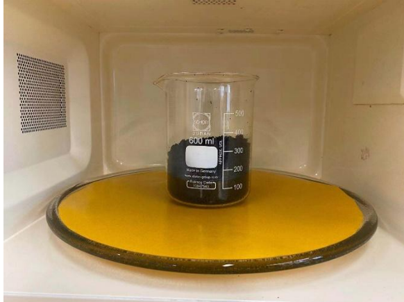
Microwave the mixtures of rubber particles and bio-oils
