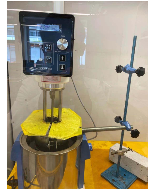
Mix the crumb rubber and base asphalt binder
