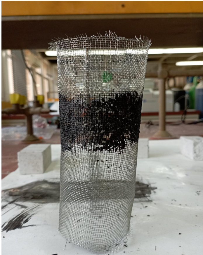
Figure 11. Si photocatalyst stabilized on stainless steel mesh using carbon paint.
