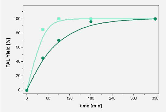
**Reaction conditions:** 120 °C, 0.25 g catalyst; 40 mL solution of furfural (0.1 M); solvent, 2-propanol;  $H_2$  or  $N_2$  pressure, 10 bar; stirring, 500 rpm; FAL, furfuryl alcohol.
