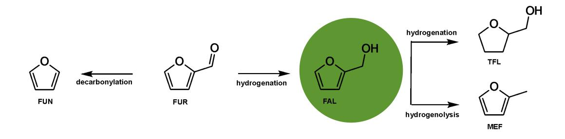
**Furfuryl alcohol** is also the chemical substrate in the production of tetrahydrofurfuryl alcohol, levulinic acid, pentane diols and precursor molecules for many materials and pharmaceutical intermediates
