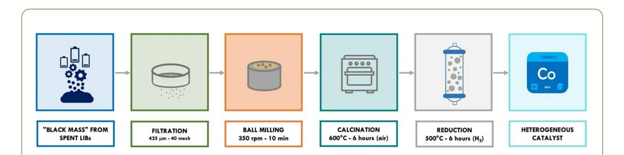
After a first **ball milling process (350 rpm for 10 min)**, the milled sample was filterd by using a sieve screen mesh (425 μm - 40 mesh) and **calcined under atmosphere conditions at 550°C** for 6 hours. Before catalytic tests, BM was finally reduced at 500 °C for 6 hours under H<sub>2</sub> flow (1 mL/min)
