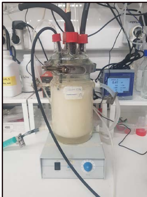
LAB-SCALE ACIDOGEN CSTR (V= 1.1 L; pH= 5.5; T= 29 ± 1 °C)
