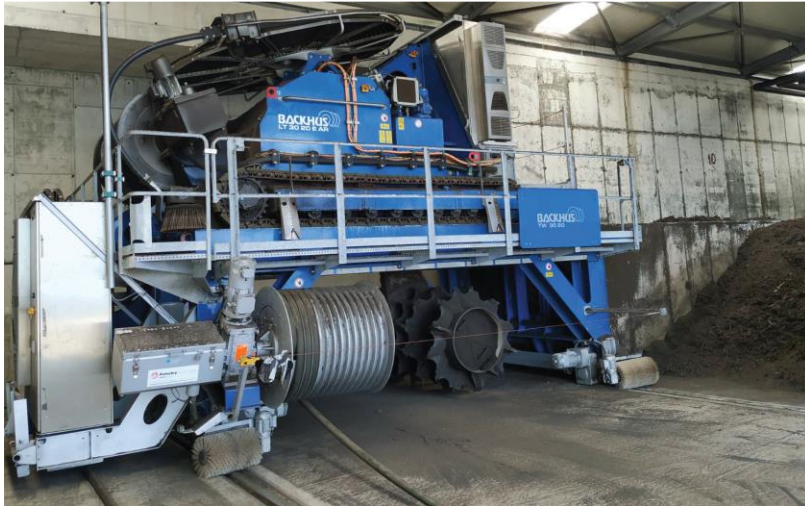
Picture 05: Mechanical stirring and promotion of the mixture
