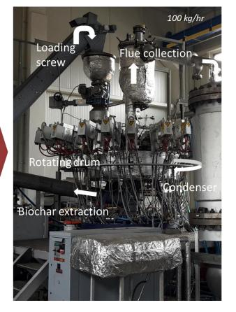
**Pyrolysis:** sludge subject to high temperature (350–600 °C) in the absence of  $O_2$ . Converted into biochar, pyrolysis oils, water vapor, and combustible gas in varied proportions.
