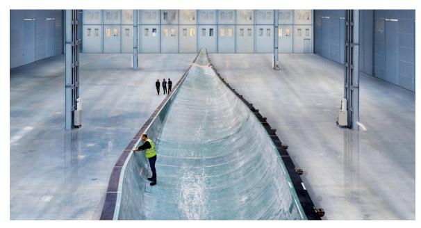
Siemens B75 blade in its mould.
