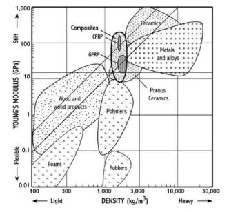
**Figure 4** Diagram showing stiffness versus density for all materials. The merit index for a beam  $M_b = E^{\frac{1}{2}}\rho$  is represented by sloping lines with  $M_b$  equal to 0.003 (*lower line*) and 0.006 (*upper line*). The criterion for absolute stiffness E = 15 GPa is indicated by the horizontal line (4).
