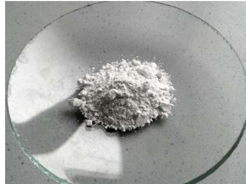
PHA extracted by aqueous inorganic reagents
