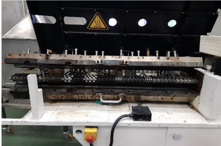
APV Baker extruder used for producing dog food kibbles
