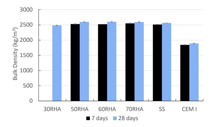
Bulk density values were like control paste and higher than those obtained for Portland cement specimens.
