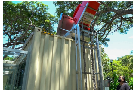
Food waste loading system
