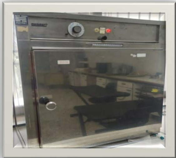
Convective Air Dryer ( Memmert, model U40 791 450, Western Germany ) Power: 2000 W
