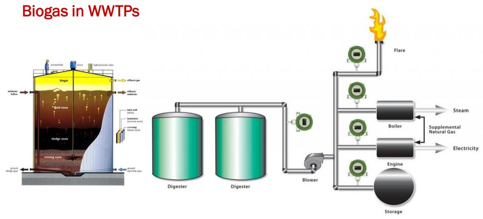
Production of heat and electricity usually via cogeneration
