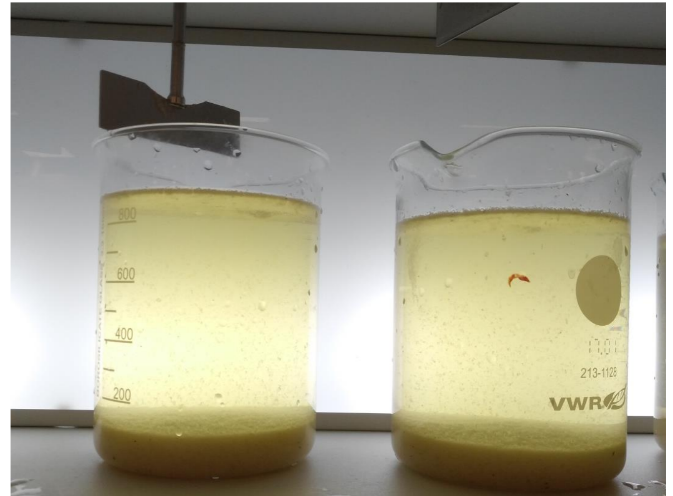
Faecal sludge coagulated with \text{AlCl}_3 (dosage: 150mg/g TS)
