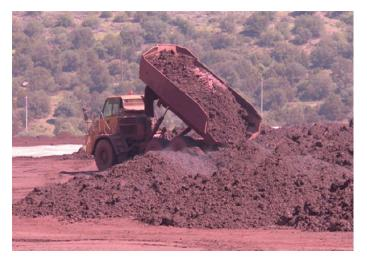
Filter-pressed (dry) bauxite residue being stockpiled in Greece, at Mytilneos S.A. (former Aluminum of Greece)
