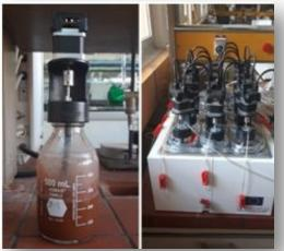
Automated Methane Potential Test System II (AMPTS)
