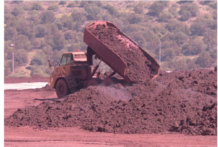
*Filter-pressed (dry) bauxite residue being stockpiled in Greece, at Mytilneos S.A. (former Aluminum of Greece)*
