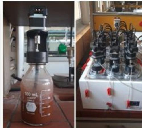
*Automated Methane Potential Test System II (AMPTS)*
