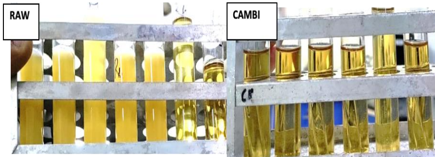
Fecal coliform analysis of raw and CAMBI pretreated sludge.
