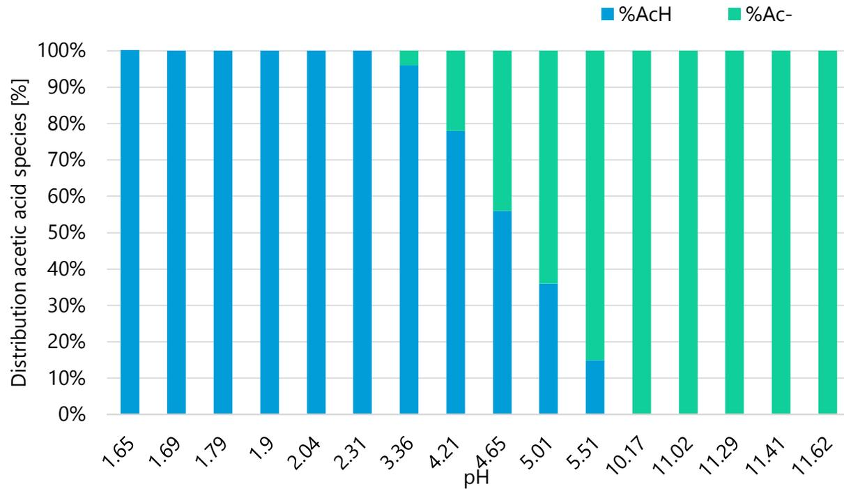
Fig 3. Acetic acid (AcH) and acetate (Ac-) equilibrium in a synthetic hydrolysate.
