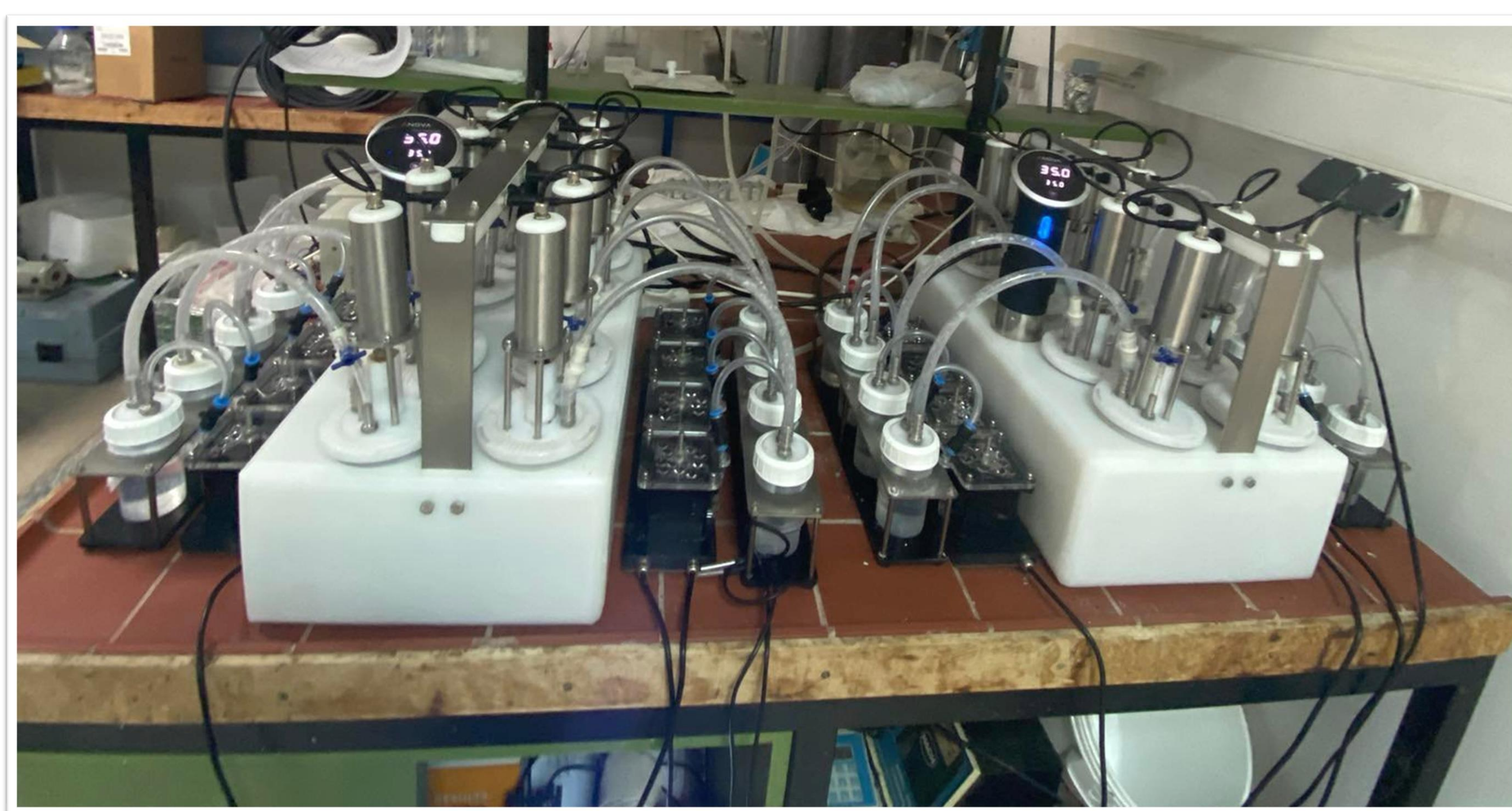
Figure 1: Experimental set up for Anaerobic Digestion and Biomethane Potential Tests
