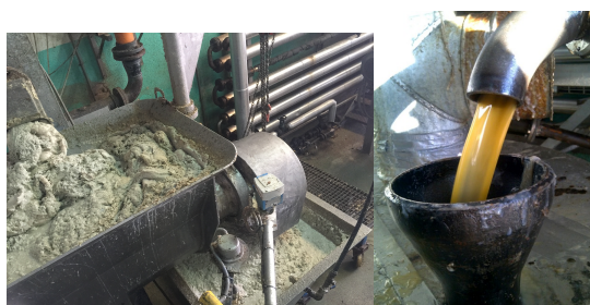
Figure 1. Separating process of the fleshing into fat and protein fractions (images courtesy of Organovac).
