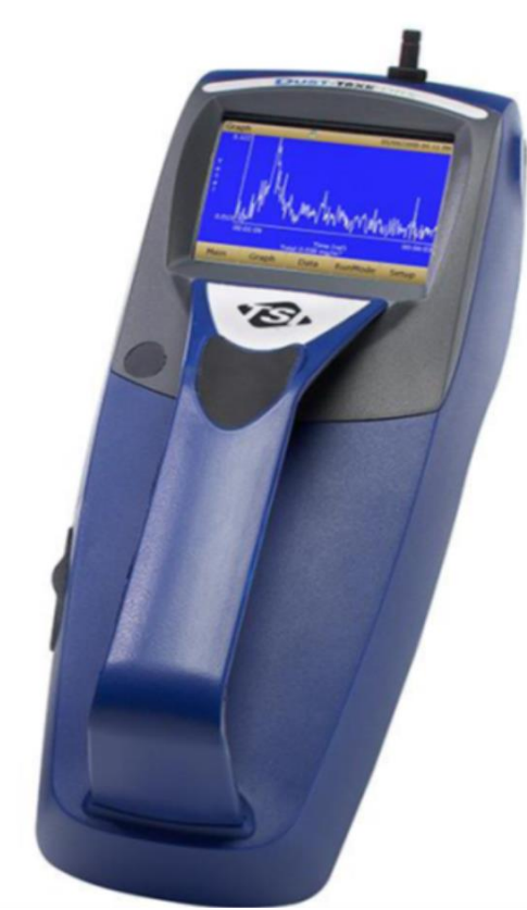
Figure 2. Portable particulate matter meter - Dust Trak Model 8532.
