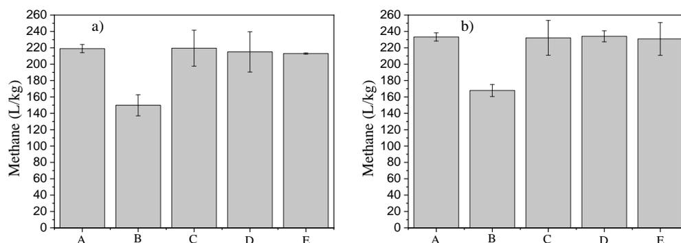
Figure 1: BMPs of a) willow sawdust (WS) and b) date palm fiber (DPF)
