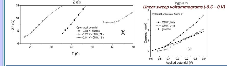
✓ The open circuit potential (OCP) value decreased from -0.568 V (glucose) to -0.507 V (OMW, 24 h) and -0.441V (OMW, 18 h)
