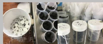
Fig. 3: Cartridges for measurement of the sanitation potential
