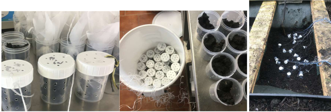
Figure 1. The two types of cartridges with artificially-added E. coli – allowing and not allowing for earthworm activity, and the on-site installation process
