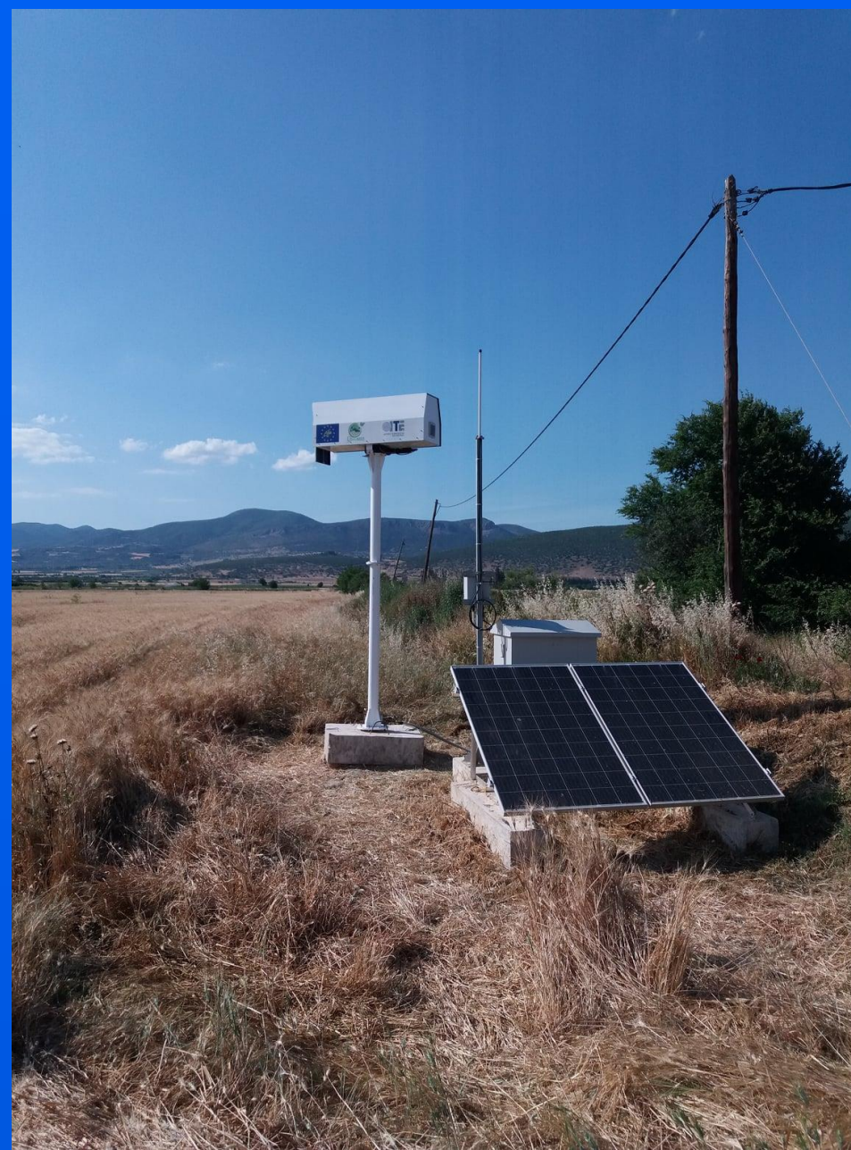
Figure 1: LIDAR device installed at a pilot field
