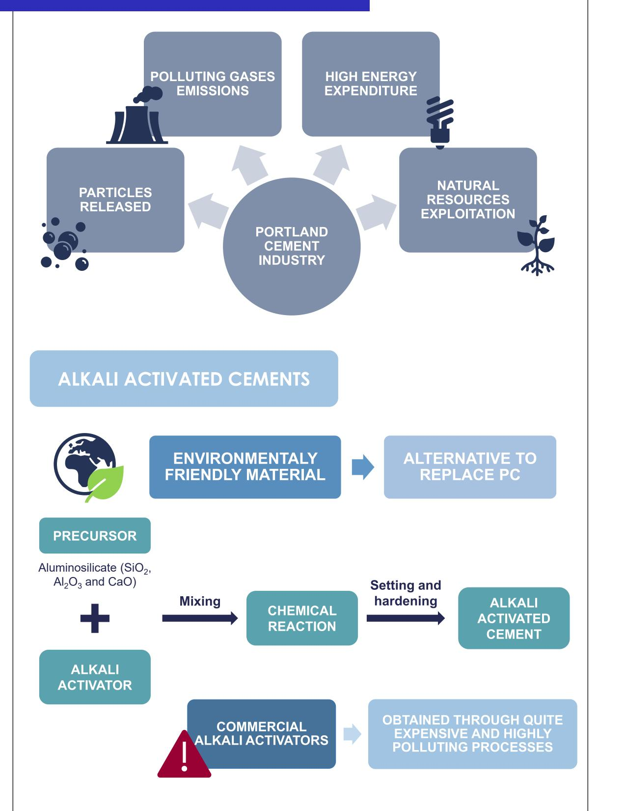
The purpose of this work was to investigate the possibility of using olive pomace fly ash (OPA) as alternative alkali activator to produce copper slags (CS) based alkali activated cements.
