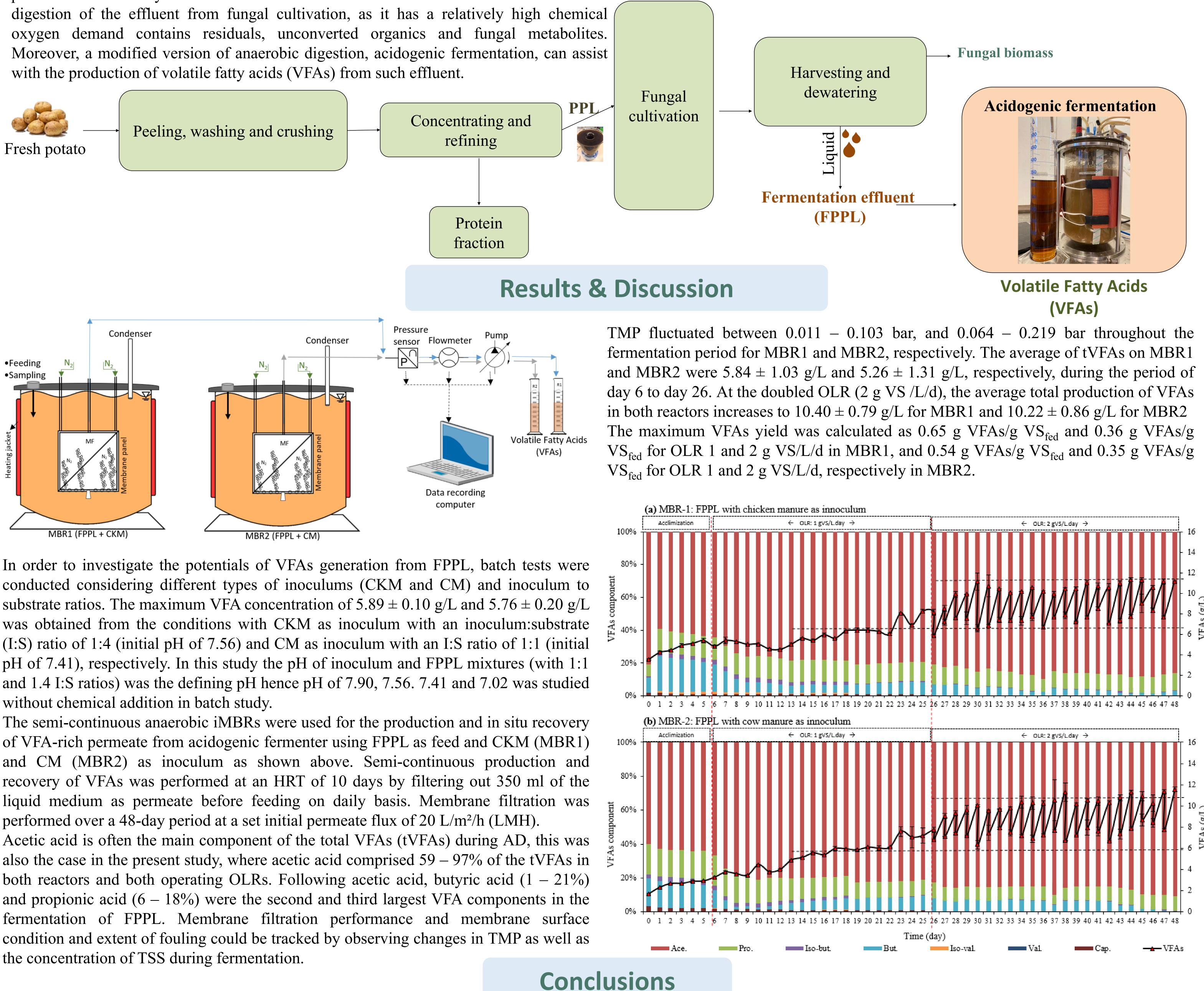
of VFA-rich permeate from acidogenic fermenter using FPPL as feed and CKM (MBR1) recovery of VFAs was performed at an HRT of 10 days by filtering out 350 ml of the performed over a 48-day period at a set initial permeate flux of 20 L/m<sup>2</sup>/h (LMH). the concentration of TSS during fermentation.
