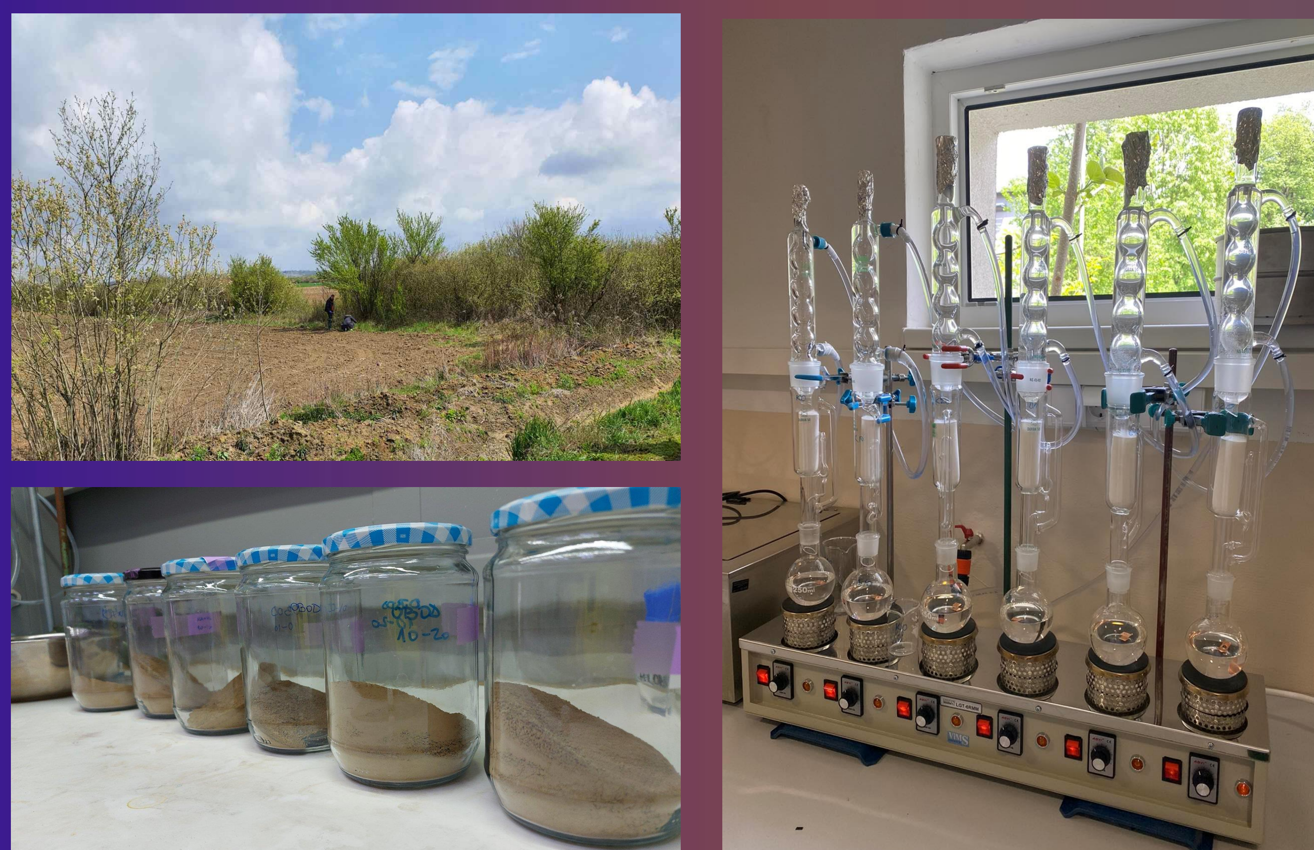
Figure: Sampling, sample preparation and extraction of specific biomarkers of the presence of pollutants on the tested soils
