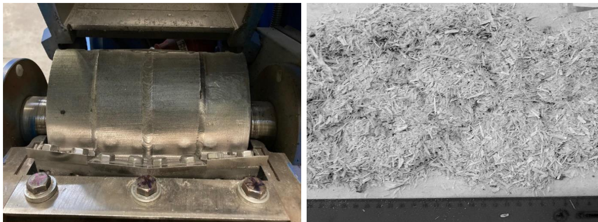
Fig. 5 Shear mill CM 2500 (left), crushing output (right)
