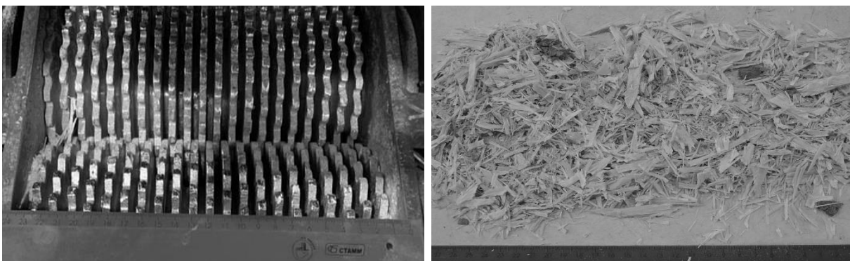
Fig. 3 Double-shaft shredder DR120, (left), crushing output (right)
