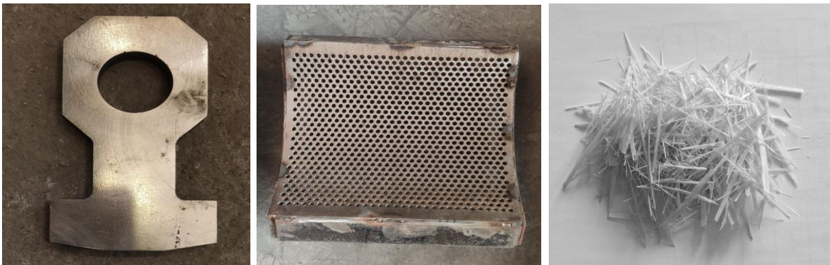
Fig. 2 Hammer shredder RTZ: hammer part (left), grate (middle), crushing output (right)
