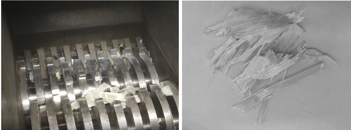
Fig. 4 Double-shaft shredder DRK500 (left), crushing output (right)
