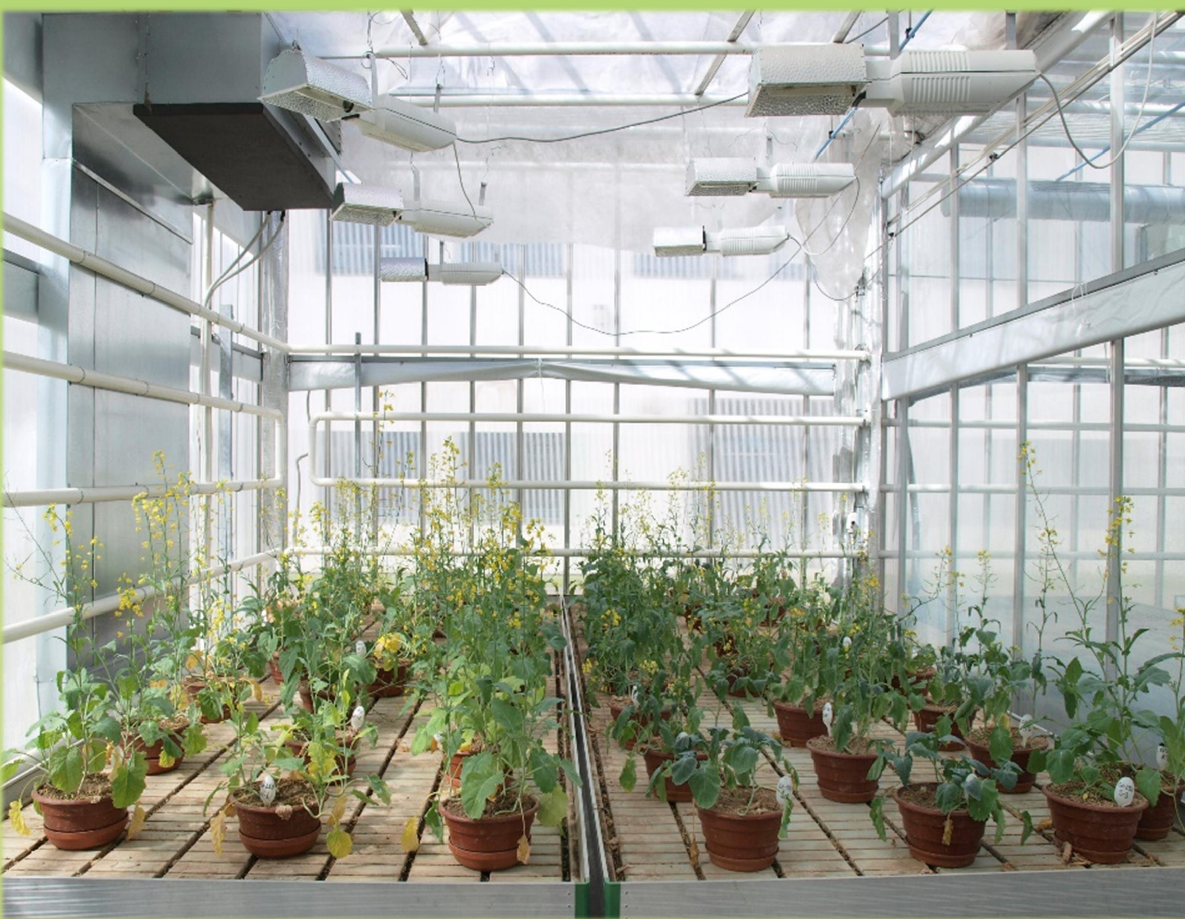
Picture 1: mesocosm experimental site of Cd phytoextraction using summer rape.
