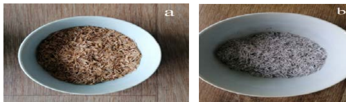
Fig. 1 Photos of rice husk: a) raw and b) oxidized
