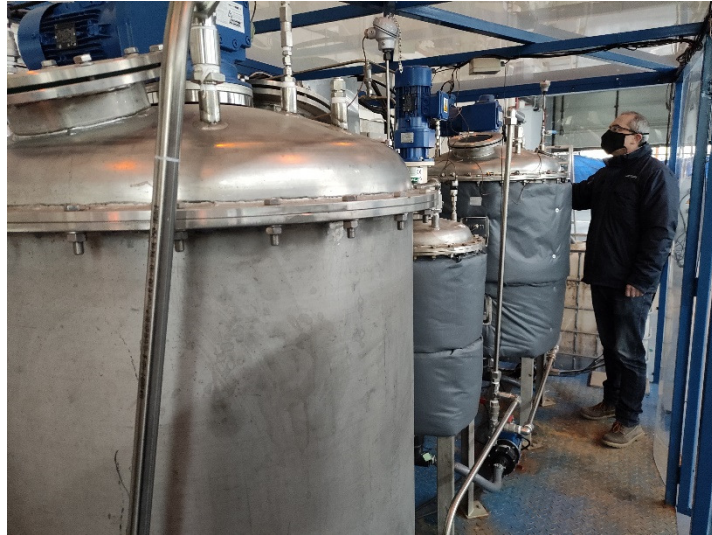
Figure 1. Pilot plant for biohydrogen production by dark fermentation
